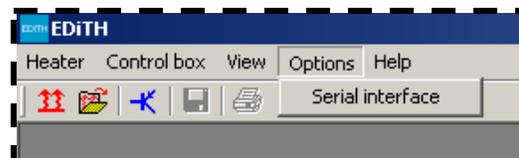
In the selection box that appears, select the communications port that corresponds to the port in which the ISO adapter is connected (White Box).
